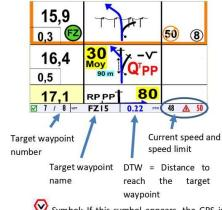
Symbol: If this symbol appears, the GPS is checking the max speed
